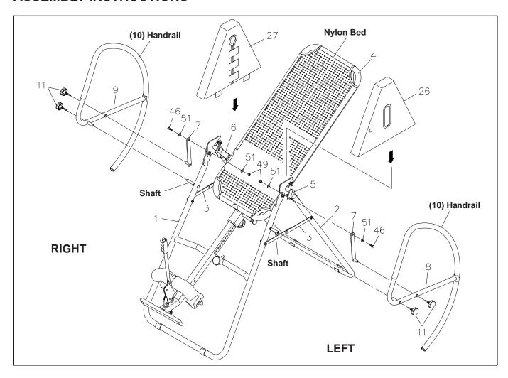
STEP 10: Slide the LEFT and RIGHT PROTECTIVE COVERS(26, 27) onto each side of the BASE ASSEMBLY. Make sure the SHAFTS on the FRONT FRAME(1) poke out through the hole on the PROTECTIVE COVERS(26, 27).
